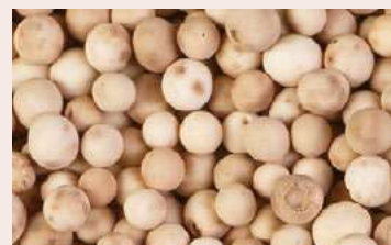
Bottom Layer - Polishing Molecular Sieve
