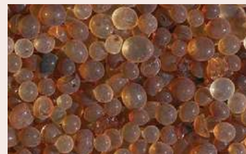
Middle Layer - Bulk drying Silica Gel
